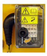
Operate a hoisting movement at the third notch; the frequency converter must stop it in less than 5 seconds and display the error SPF.
