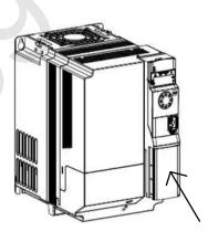
■ Disconnect the wire of the DI5 terminal from the control terminal strip.
