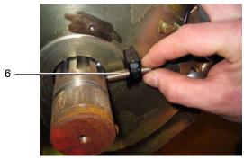
Screw in or unscrew the inductive sensor (6) in order to obtain an adjusting dimension of 0,5 mm ±0,1mm (check by means of an adjusting wedge).
