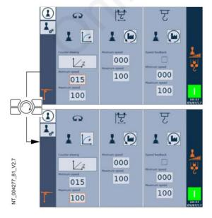
14. Use the **Jog Dial** to select the setting for the maximum speed of the slewing movement.
