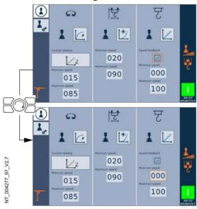
30. Use the **Jog Dial** to select the setting for the minimum speed of the hoisting movement.
