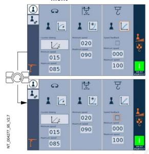
Use the Jog Dial to select the parameter for activation/deactivation of the "Speed feedback" function for the hoisting movement.
