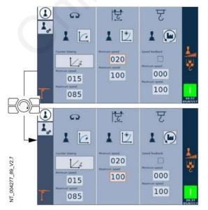
22. Use the **Jog Dial** to select the setting for the maximum speed of the trolleying movement.
