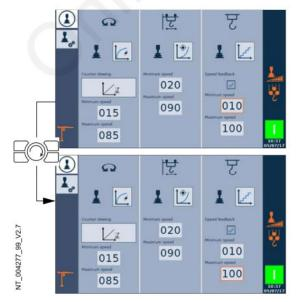
32. Use the **Jog Dial** to select the setting for the maximum speed of the hoisting movement.
