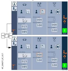
20. Use the **Jog Dial** to select the setting for the minimum speed of the trolleying movement.
