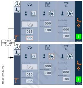
16. Use the **Jog Dial** to select the parameter for trolleying movement delinearization.
