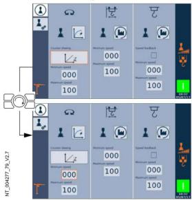
12. Use the **Jog Dial** to select the setting for the minimum speed of the slewing movement.
