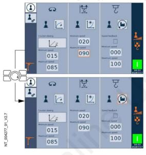
24. Use the **Jog Dial** to select the parameter for hoisting movement delinearization.
