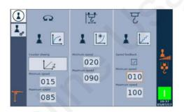
31. Enter the desired value → page 1-22 for the minimum speed of the hoisting movement → page 1-37.
