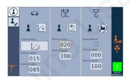
21. Enter the desired value → page 1-22 for the minimum speed of the trolleying movement → page 1-37.
