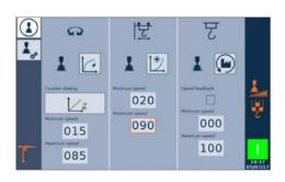
23. Enter the desired value → page 1-22 for the maximum speed of the trolleying movement → page 1-37.
