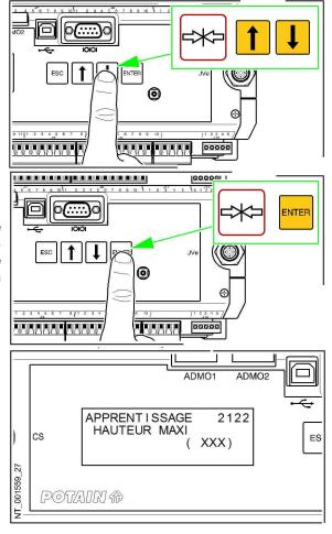
■ Lower the pulley block until 3 dead turns remain on the drum. During the lowering movement the analog value must increase and remain lower than **3500 pions**.
