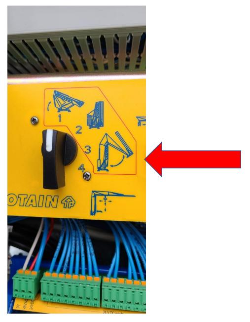
• C3 and maintenance mode (trolley out) jib goes down (go down until sensor is out of range of alignment plate -5 feet-)
