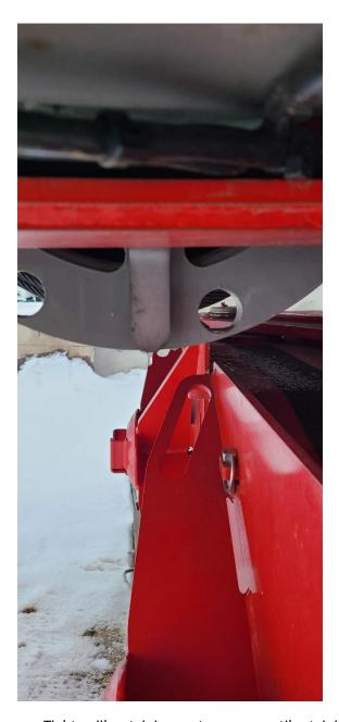
• Tighten jib retaining motor screw until retaining pin slides out.
