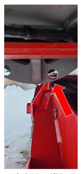
Press button to go past 2 holes, and insert pin
