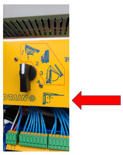
• Validate (push button at least 3 times) and switch back to C4 and honk horn
