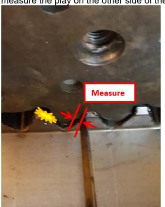
2-Or measure the play on each side of the tooth, but this must be done with two sets of shims Add the two measurements together
