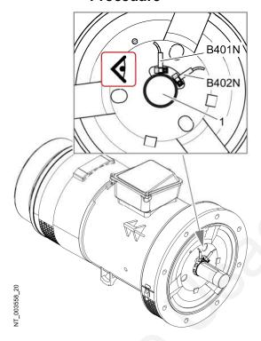
Check the air gap between the motor shaft (1) and the inductive speed sensors (B401N) and (B402N).
