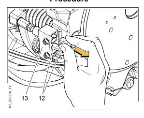
1. Disconnect the two terminals (12) on the microcontact (13).
