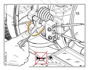
Screw in the screw (15) again until the multimeter stops ringing.
