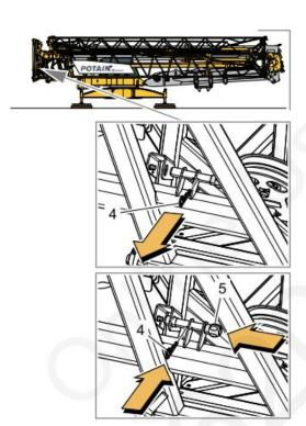
Lock the counter-jib by removing the safety pin (4), pushing in the locking pin (5) then reinserting the safety pin (4).
