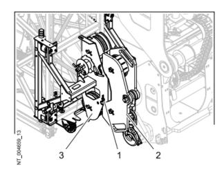
Remove pin 1 to free the pulley block
