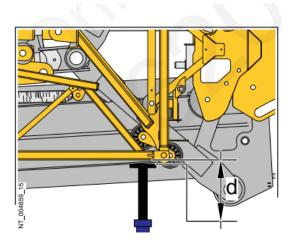
Adjust the height of the adjustable supports so that they are as close as possible to the lower members of the jib foot.
