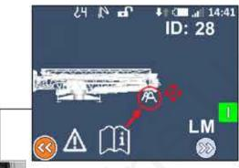
7. Confirm the presence of the adjustable supports by turning the **Jog Dial** to select **...** Press the confirmation key on the **Jog Dial**.
