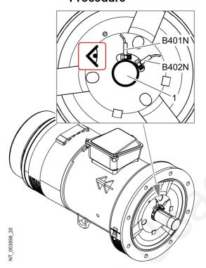
1. Check the air gap between the motor shaft (1) and the inductive speed sensors (B401N) and (B402N).
