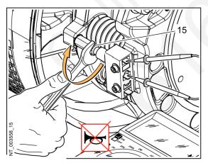
5. Screw in the screw (15) again until the multimeter stops ringing.
