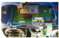
—The HF block existing in the transmitter and in the processing unit has no configuration switches. Adjusting the groups and the frequencies is done by means of the configuration menu of the transmitter and the processing unit (for GMA and MCT without shifted receiver).
