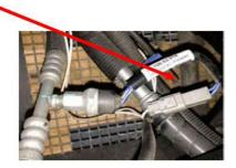
If there is no continuity at the connector of the pressure sensitive switch, this indicates a fault in the pressure sensitive switch or a unit without gas, which prevents the air-conditioning system from functioning.
