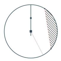
An open prohibited zone is one where the edges of the zone are located on the maximum slewing radius of the jib (trolley at jib nose).
