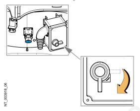
13. Turn the crane's isolating switch ON.
