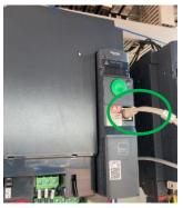
5. Remove the plug to install the Can Open card.
